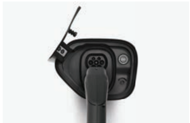
Insert the charging plug into the car's charging port (maximum 4 meters from the Two).
